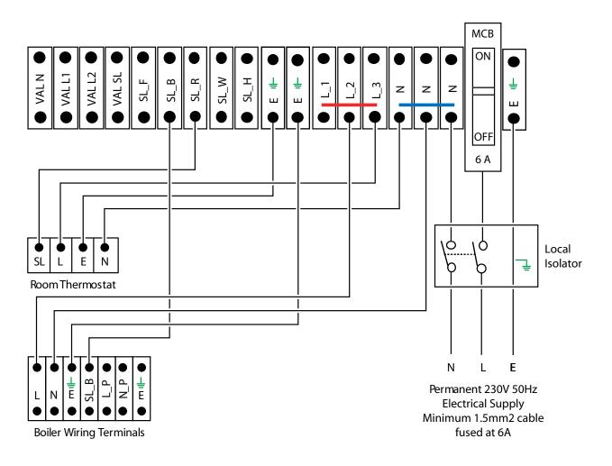
If frost protection is provided the existing switched live output from the frost thermostat should be connected into the SL-F terminal provided.
