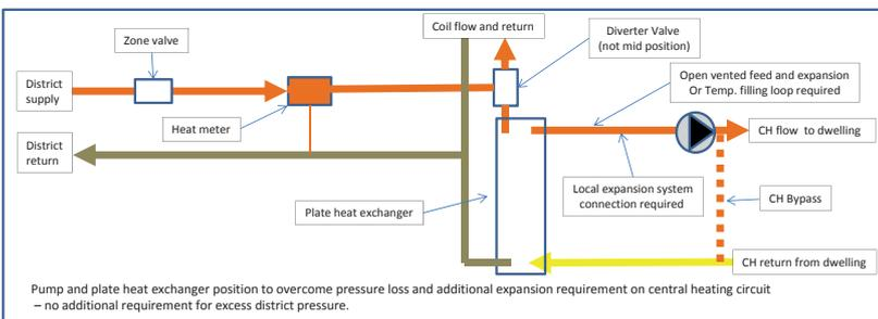
Here, the plate heat exchanger has been fitted because the expansion requirements of the central heating system are to be handled in the dwelling rather than the whole system, or the components in the central heating system are not capable of withstanding the pressure of the district heating system.
