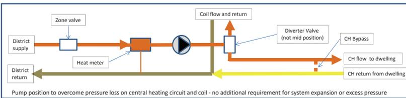
The pump is now fitted in the district supply because the pressure loss over the BoilerMate CP coil is too large.
