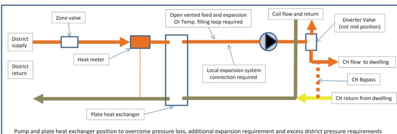
In this instance, the plate heat exchanger provides a full pressure break between the district heating system and the dwelling system. The dwelling system will need to cater for expansion and circulation requirements. This may be used where excessive district heating pressure occurs.
