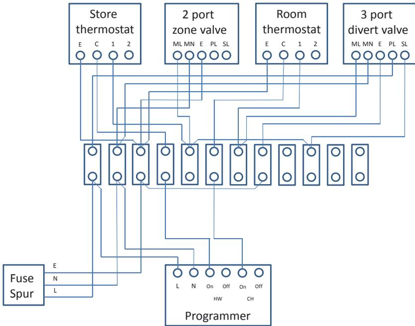
The following control wiring diagrams ensure that the district heating system is isolated from the dwelling when charging is not required.
