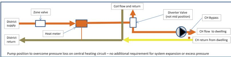
In this diagram an additional pump is shown fitted because the pressure loss in the central heating system is too large for the district pump.
