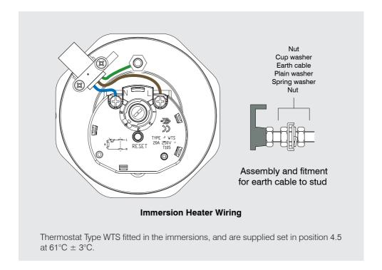
The immersion heater is supplied with a thermostat which has been tested for operation in the cylinder and complies with the European directives for Electromagnetic compatibility and radio interference. It is Rated at 20 Amp 250V ~AC.
