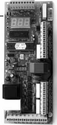
Appliance Control Board A.C.B.
